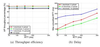
Fig. 16. Performance of the A\* algorithm as the wired RTT is varied. Physical layer data and basic rates are 54 and 6 Mbps. Here the AP throughput percentage is the ratio between the throughput achieved using the A\* algorithm and the maximum throughput using fixed size buffers.
